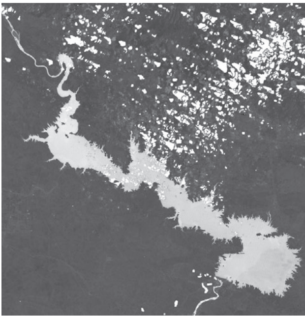
Fig. 6 - Example of missing information due to clouds and lack of enough images for the median reducer to fill missing pixels.
